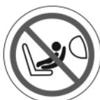
\* Backward facing child restraint systems may never be used with an activated front airbag (Fig.12)!
